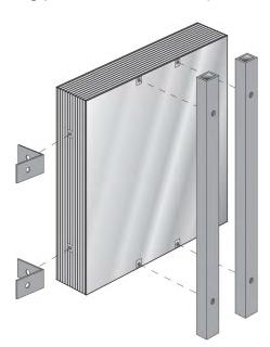
These mounting points are simple and generic enough to accommodate a variety of techniques for hanging the display on assorted structures. The rear mounting points accept 1/2-inch 13 bolts and are provided for mounting structures that can run behind the shot clock cabinet. In some cases, it may be easier to attach support pieces to the sides of the shot clock cabinets. The side mounting points accept 3/8-inch 16 bolts.
